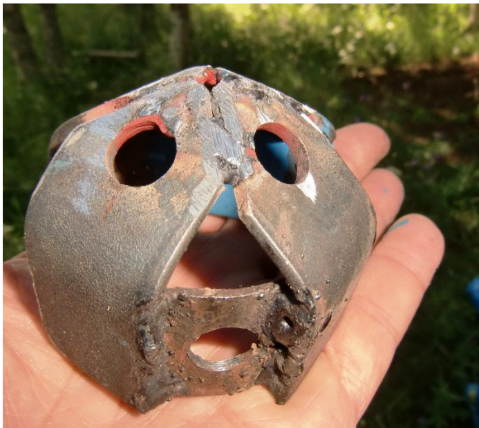
The “PET CROWN” space frame connector
