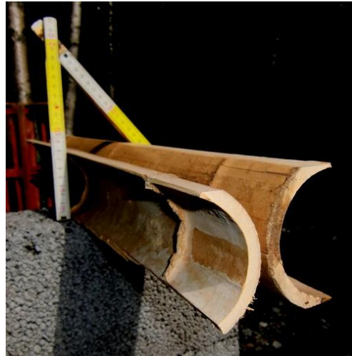
Bamboo dimensional standard: Purlin back-to-back assembly
